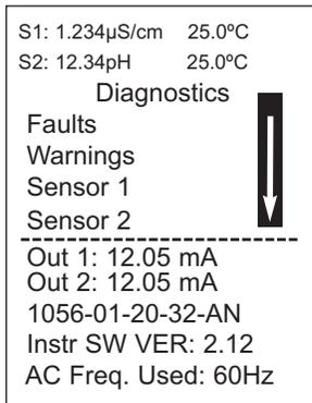
Information about each condition is quickly accessible by pressing the diagnostic button on the keypad. User help screens are displayed for most fault and warning conditions to assist in troubleshooting.
